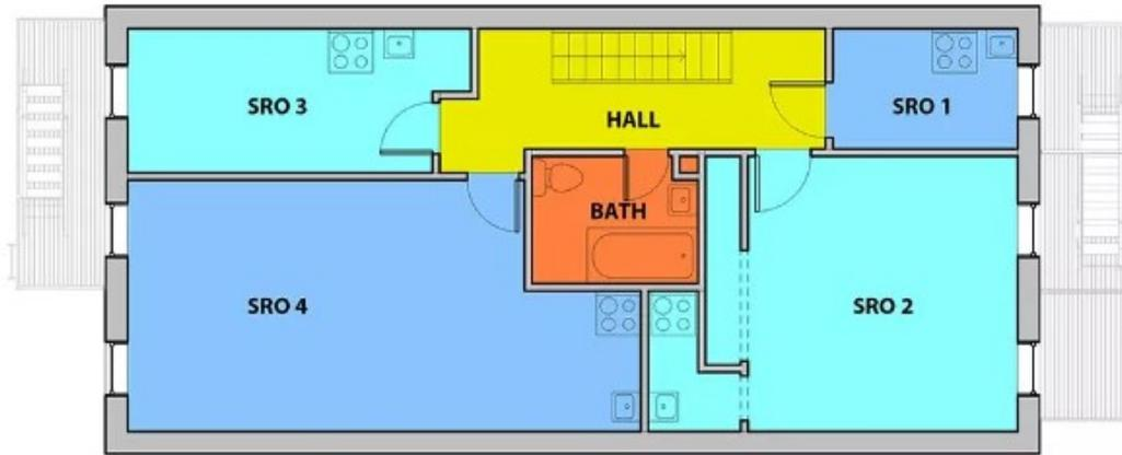
Figure 1: Proposed SRO floor plan produced by Fontan Architecture
